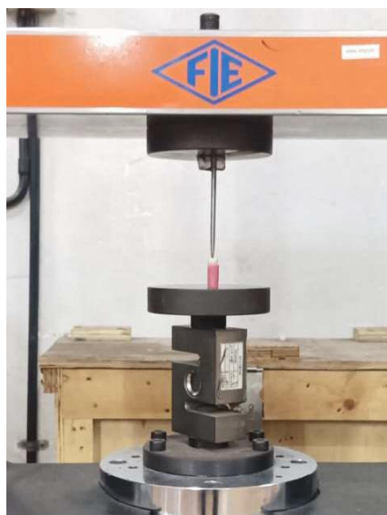
Figure 1: Fracture resistance test using Universal testing machine.
