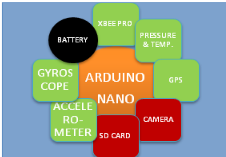
Fig 11: Communication System Overview
