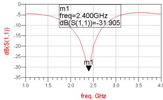
Fig.4 Return loss for Hybrid coupler
