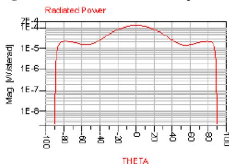
Fig.12 Radiated power of Microstrip antenna
