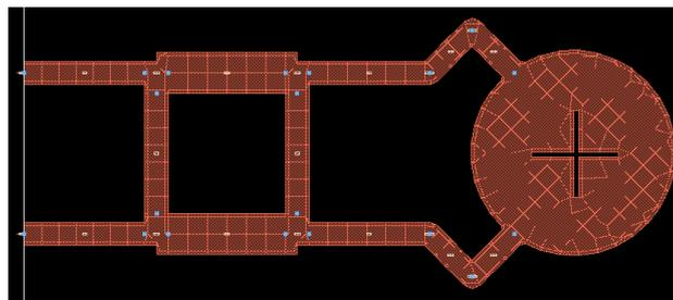
Fig.5 Proposed Antenna Layout design in ADS2009
