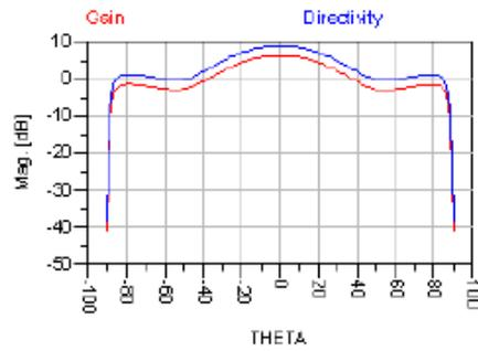
Fig.9 Gain and Directivity of Proposed Microstrip antenna
