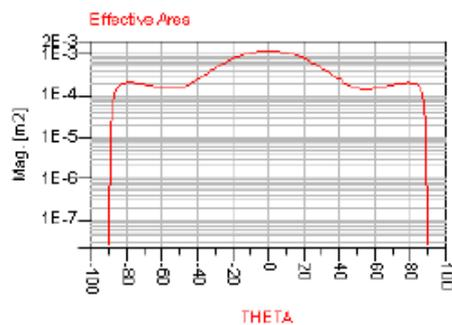
Fig.11 Effective Area of Microstrip antenna
