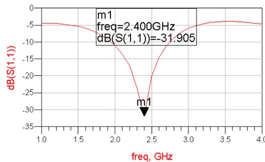
Fig.4 Return loss for Hybrid coupler
