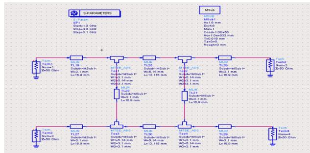
Fig.3 Schematic diagram of 3dB hybrid coupler in ADS
