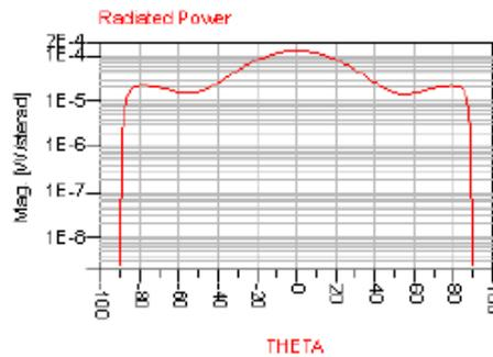
Fig.12 Radiated power of Microstrip antenna
