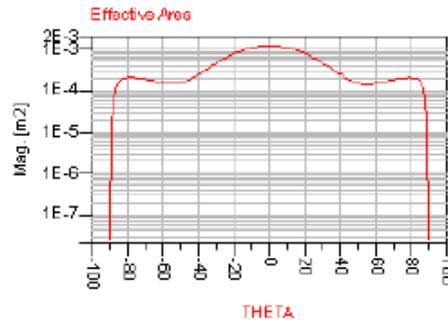
Fig.11 Effective Area of Microstrip antenna
