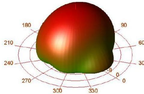
Fig.8 3D Radiation Pattern of Patch Antenna
