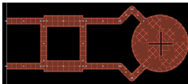
Fig.5 Proposed Antenna Layout design in ADS2009
