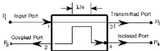
Fig. 2 Internal diagram of 3dB quad hybrid coupler
