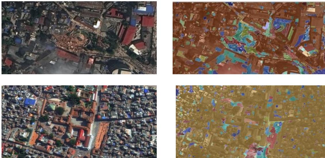
Figure.7: Structurally damaged regions marked and superimposed over the original image
