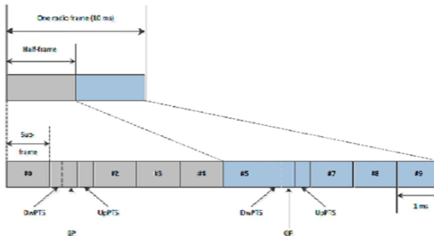
Figure 2 Type-2 LTE Frame Structure
