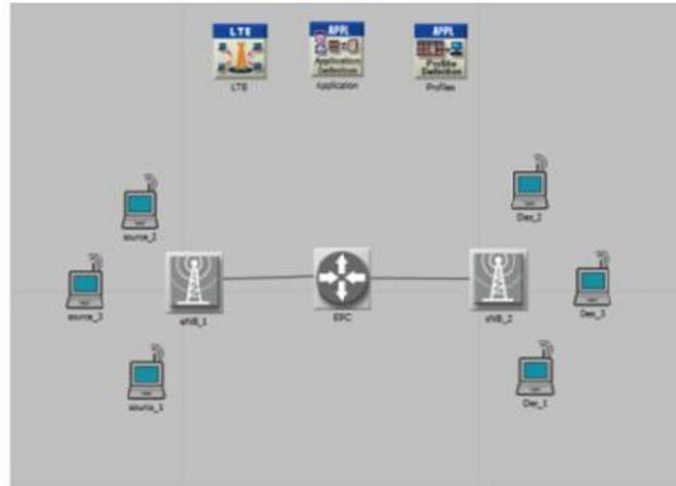
Figure 3 Network Scenario for LTE 1.3MHz
