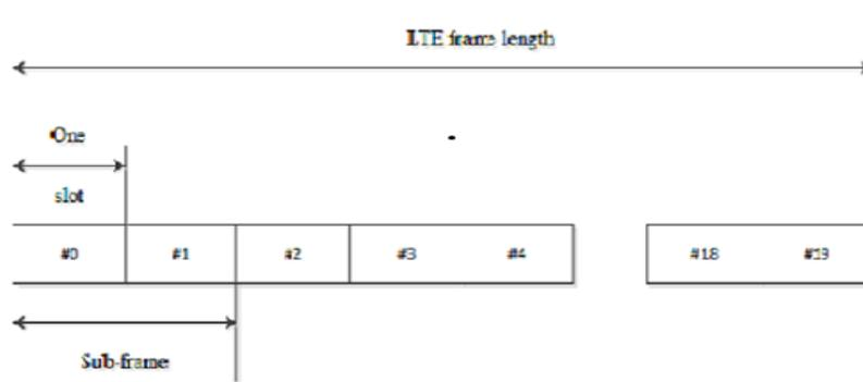
Figure 1 Type-1 LTE Frame Structure
