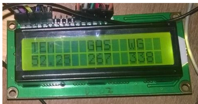
Fig 5: LCD showing output of Temperature, gas level and weight
