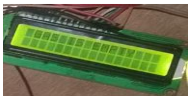
Fig 6: Output showing Status of LPG cylinder
