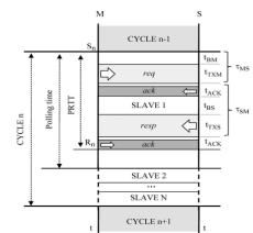
Fig 5: Time diagram of the master and slave communication.
