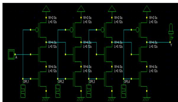
Figure 10: 4 NOT cascaded in OPL domino logic
