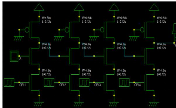
Figure 9: 4 cascaded NOT in OPL pseudo NMOS logic
