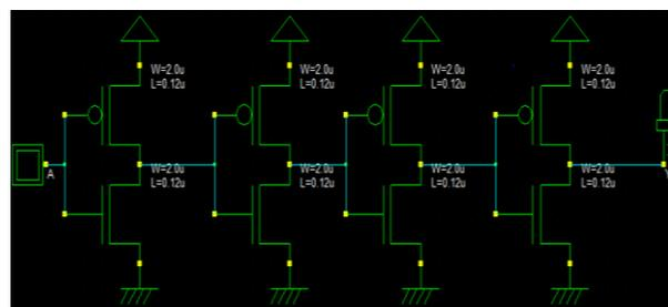
**Figure 5:** schematic of 4 NOT in static CMOS logic
