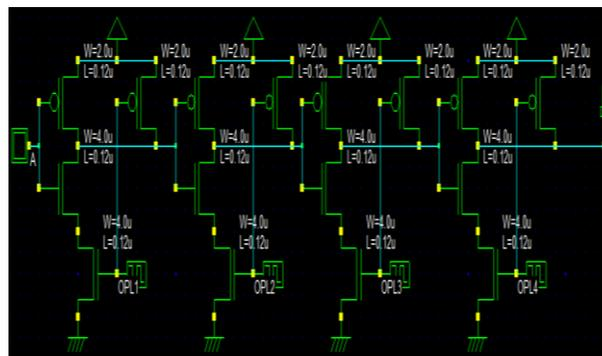
**Figure 6:** chain of 4 NOT using OPL static CMOS
