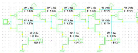
Figure 3: a chain of 3 OPL static inverters
