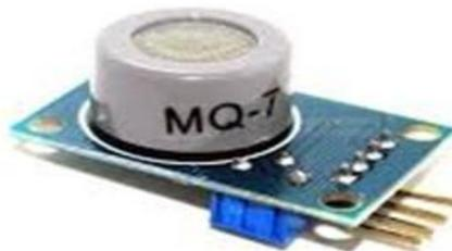
Fig 3.6 MQ7 Sensor
