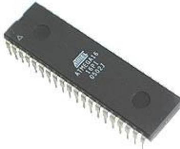
Fig 3.5 ATmega16 Microcontroller
