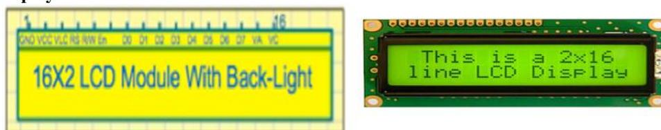
Fig 3.7 LCD Display
