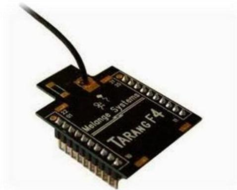
**Fig 3.8** ZigBee Transceiver Model
