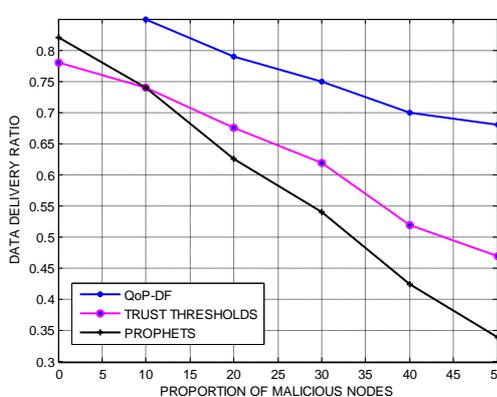
Fig. 3: Data delivery ratio under different proportions of malicious nodes.
