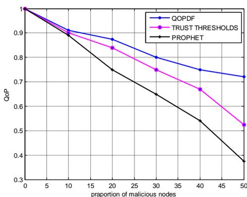
Fig. 2: The QOP under different proportions of malicious nodes
