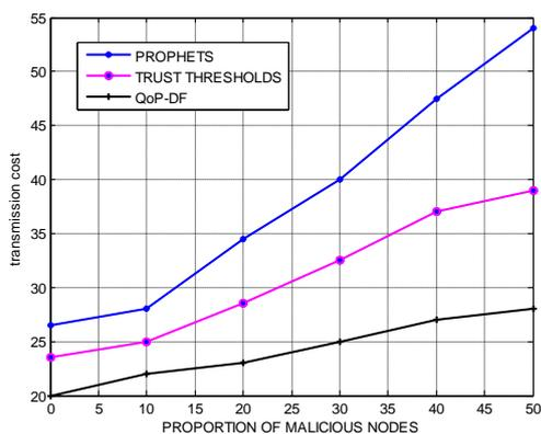
Fig. 4: Transmission cost under different proportion of malicious nodes.
