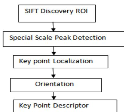
Fig1: SIFT detection model
