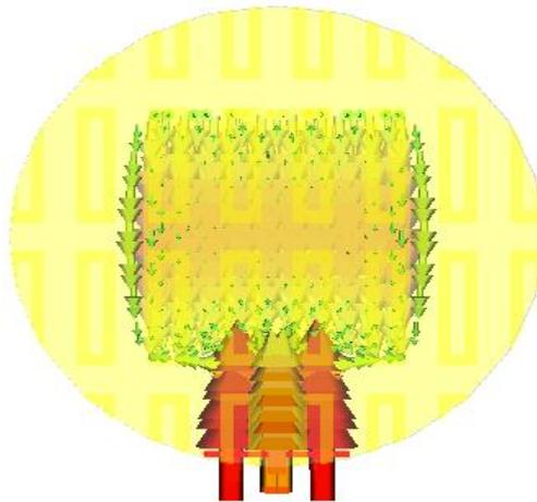
Figure 6. Surface Current of the Antenna with Metasurface.
