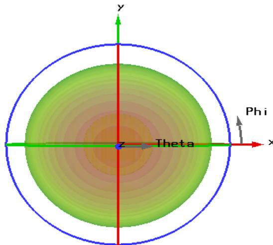
Figure 5. Far Field Radiation in Theta Direction.
