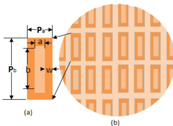
Figure 2. Geometries of (a) Unit cell and (c) Metasurface.
