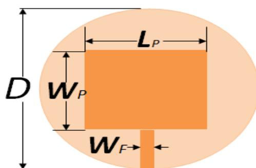
Figure 1. Geometries of Patch Antenna (source antenna).
