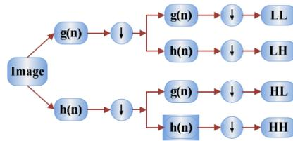
Fig.2: Schematic of 2D DWT
