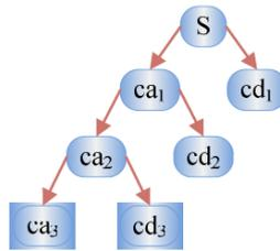
Fig.3: Wavelet decomposition at 3-level
