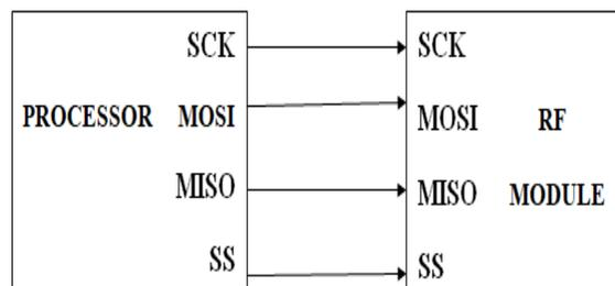
Interfacing between processor and RF module
