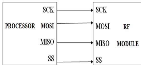
Interfacing between processor and RF module
