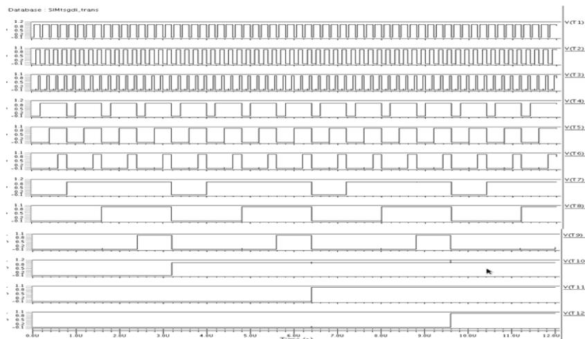
Fig.4 8-Bit Segmented BT Decoder output
