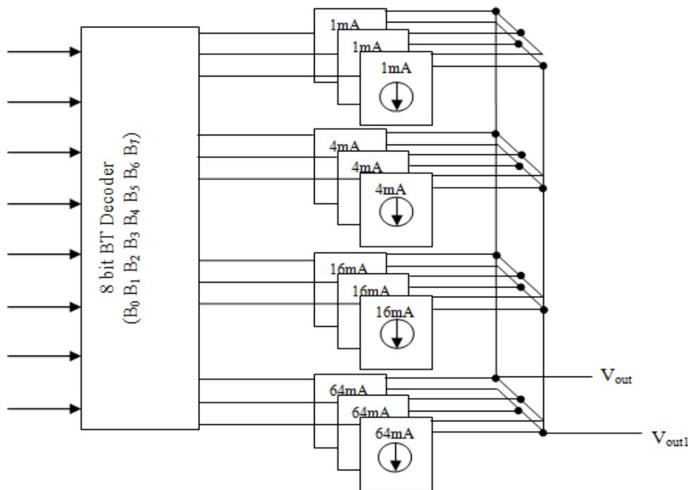
Fig. 1 8-bit Current steering DAC
