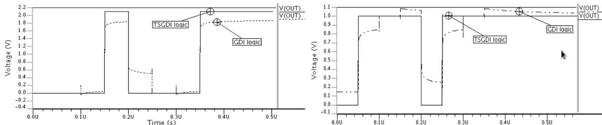
Fig. 3 output of (a) OR gate (b) AND gate using GDI and TSGDI logics
