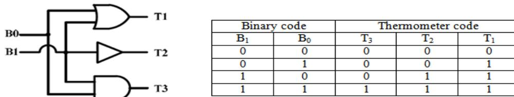
Fig.2 2-Bit BT Decoder and its operating procedure
