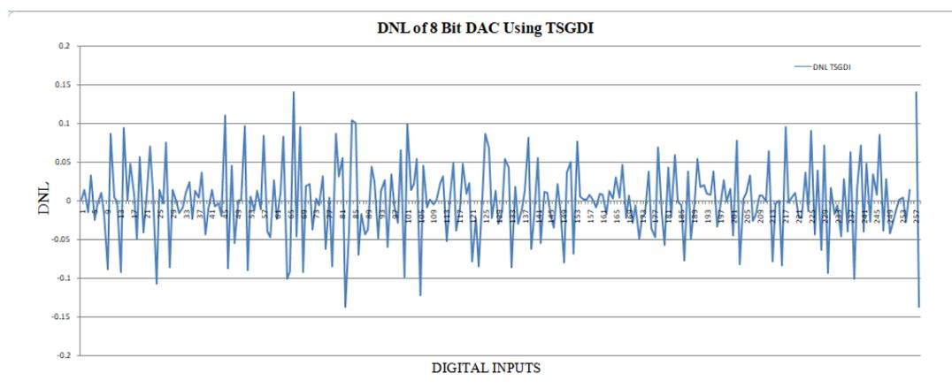
Fig.8 DNL of 8-Bit CSDAC Using TSGDI Logic
