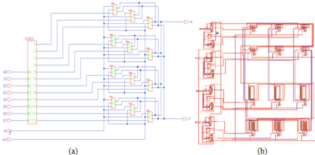
Fig.6 (a) 8-bit CSDAC Schematic and (b) Layout of 8-bit CSDAC
