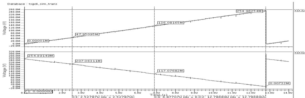
Fig.7 Output of 8-bit Current Steering DAC
