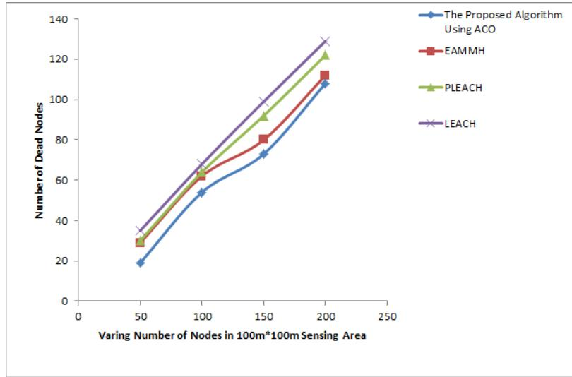
**Figure 4 : Number of Dead Nodes for Varying Number of Nodes in 100m\*100m sensing Area**
