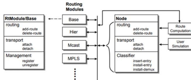
Fig 2. Interaction among node, routing module, and routing. The line shows the most points of one routing module [2]
