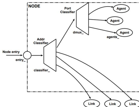
Fig 3. Structure of a Unicast Node. Notice that entry\_ is just a label variable rather than a true object [2]
