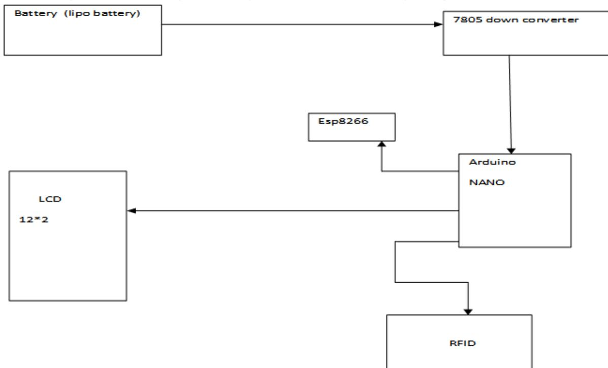
(b) **Functional diagram-** the functional diagram of our system is given below
