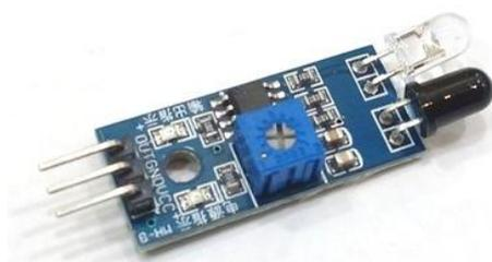
Fig 6. Shows infrared sensor
