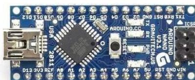
Fig 4. Shows Arduino Nano Atmega 328P
