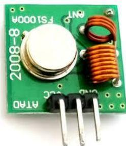
Fig 7. Shows the RF Module for transmission purpose.
