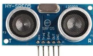
Fig 5. Shows ultrasonic ranging sensor
