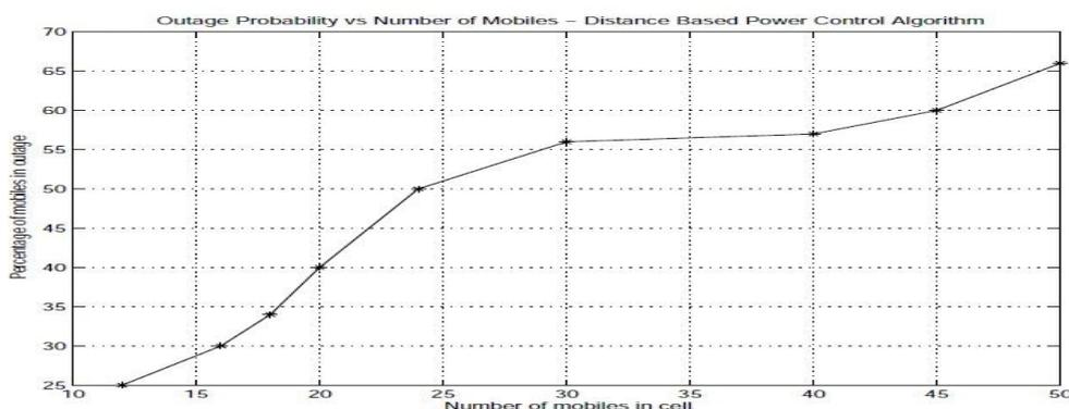
**Figure 1:** Outage probability of Distance Based Power Control Algorithm
