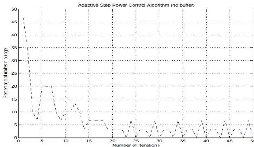
Figure 3: Outage probability of Adaptive Step Power Control Algorithm
