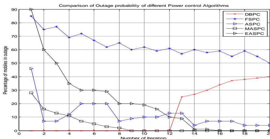
**Figure 6:** Comparison of Outage probability of the various power control techniques considered in this work
