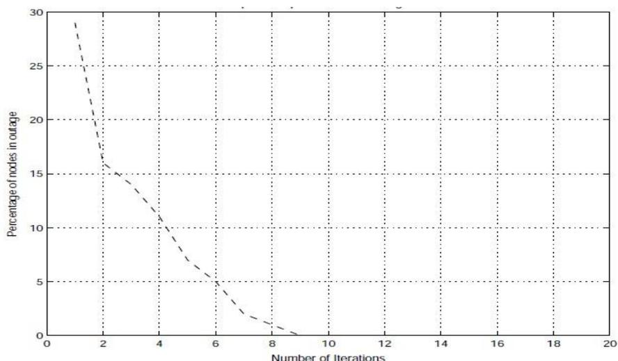
Figure 4: Outage probability of Modified Adaptive Step Power Control Algorithm
