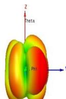
Fig. 12 Radiation Pattern When Right switch ON
