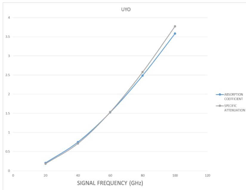
Figure 3: Graph plot of specific attenuation and absorption coefficient against frequency for the location of Uyo
