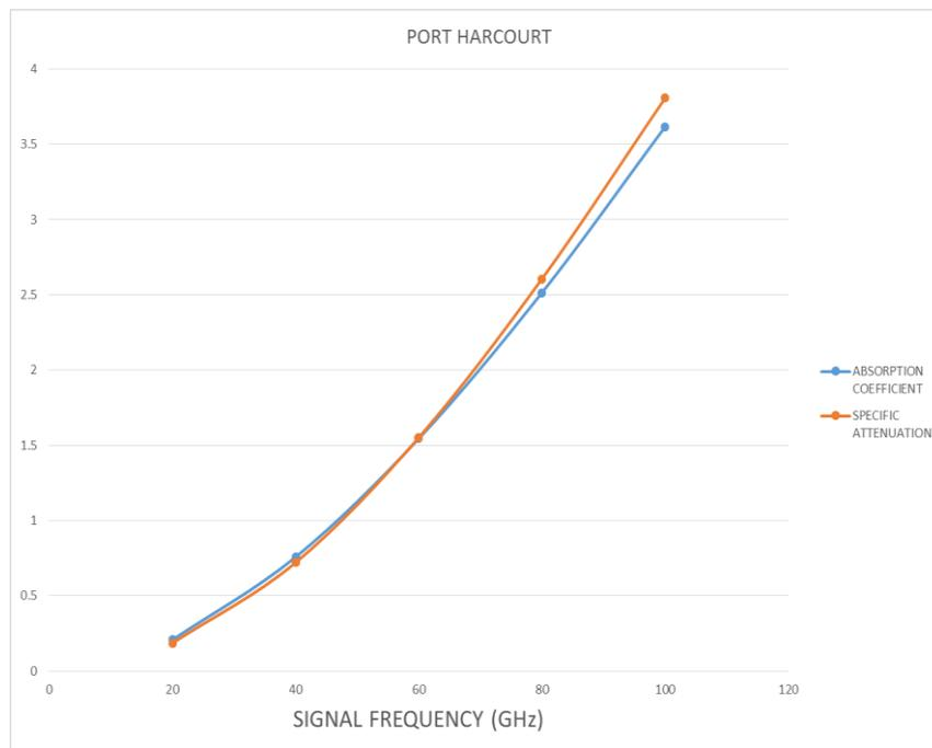
**Figure 1: Graph plot of specific attenuation and absorption coefficient against frequency for the location of Port-Harcourt**
