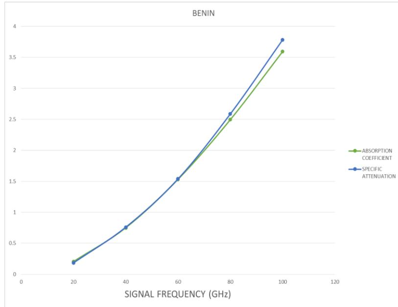
Figure 2: Graph plot of specific attenuation and absorption coefficient against frequency for the location of Benin
