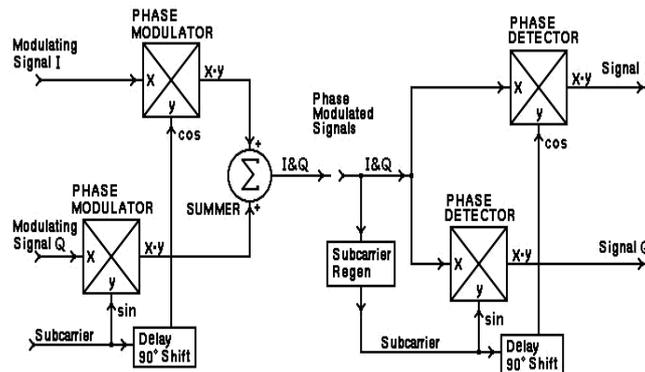
Fig 6 : Block diagram for a QAM Transmitter and Receiver.
