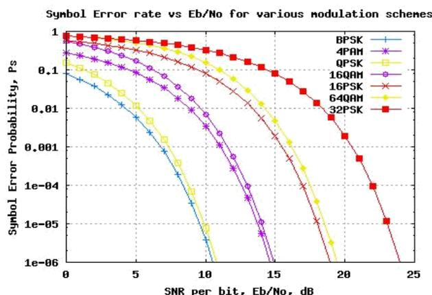
Fig 11: Theoretical SNR vs BER curves for various Modulation Schemes
