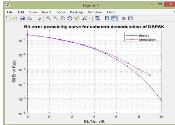
**Fig 8: SNR vs BER curve for BPSK Modulation Scheme**
