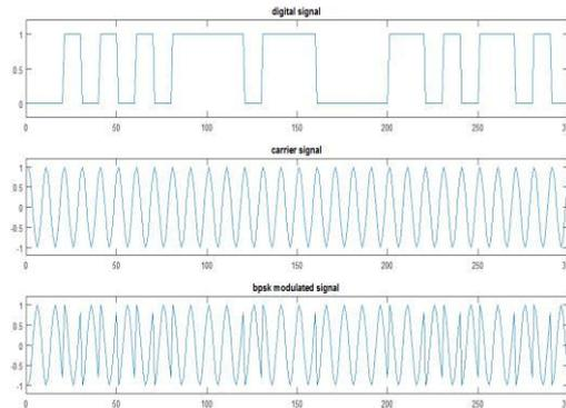
Fig 3: BPSK output for a Random Sequence
