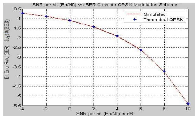
**Fig 9: SNR vs BER curve for QPSK Modulation Scheme**
