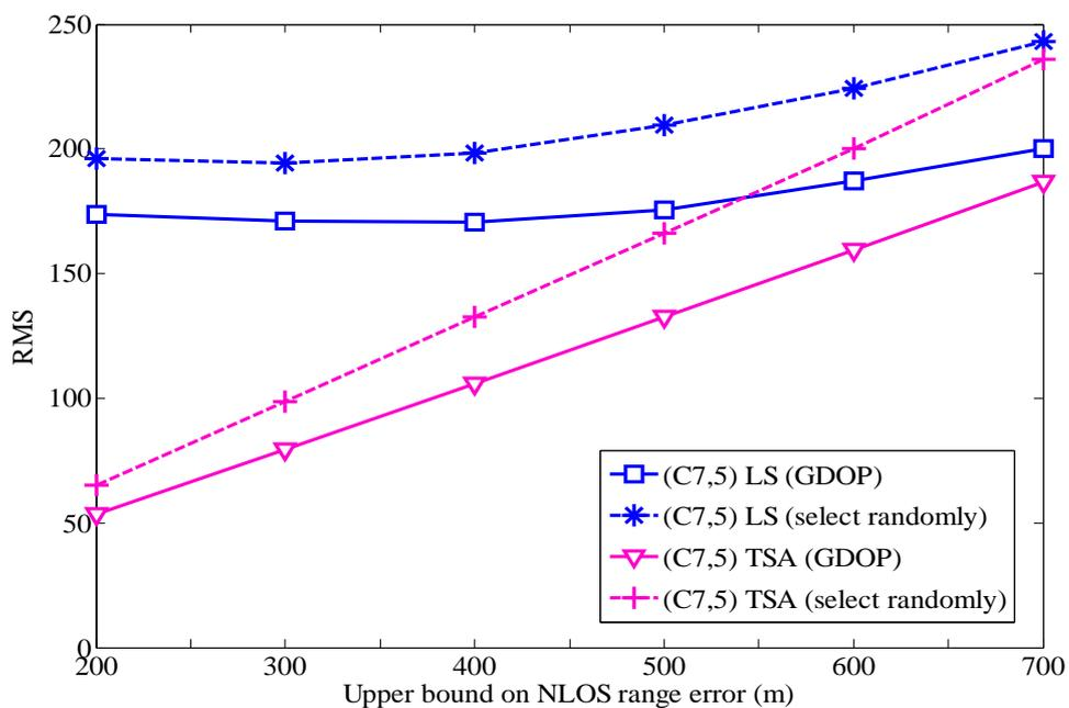
Fig. 6. Performance comparison between the location estimation methods when the upper bound is used to model the NLOS.
