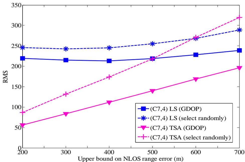
Fig. 5. Average location error versus the upper bound of NLOS errors.
