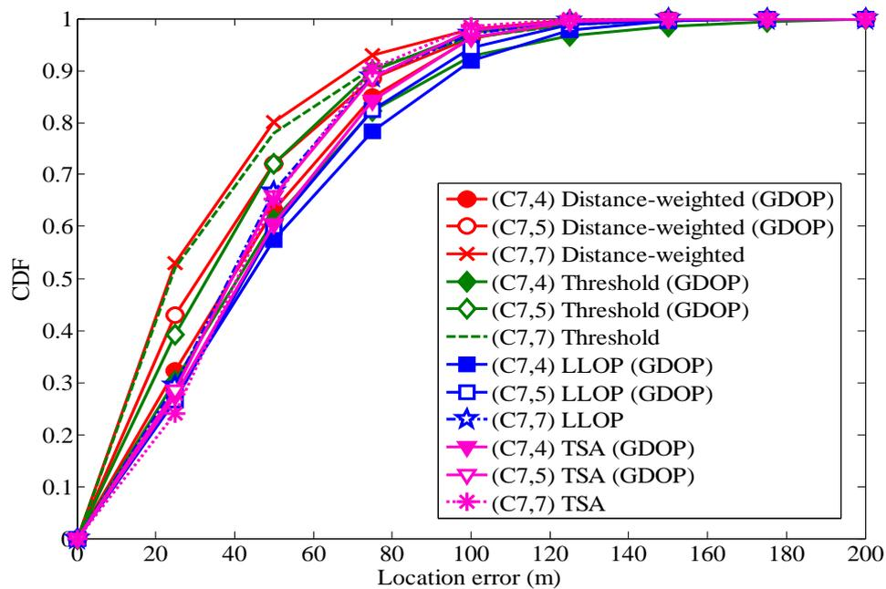
**Fig. 4.** Comparison of location error CDFs using all seven BSs and the subset with minimum GDOP.
