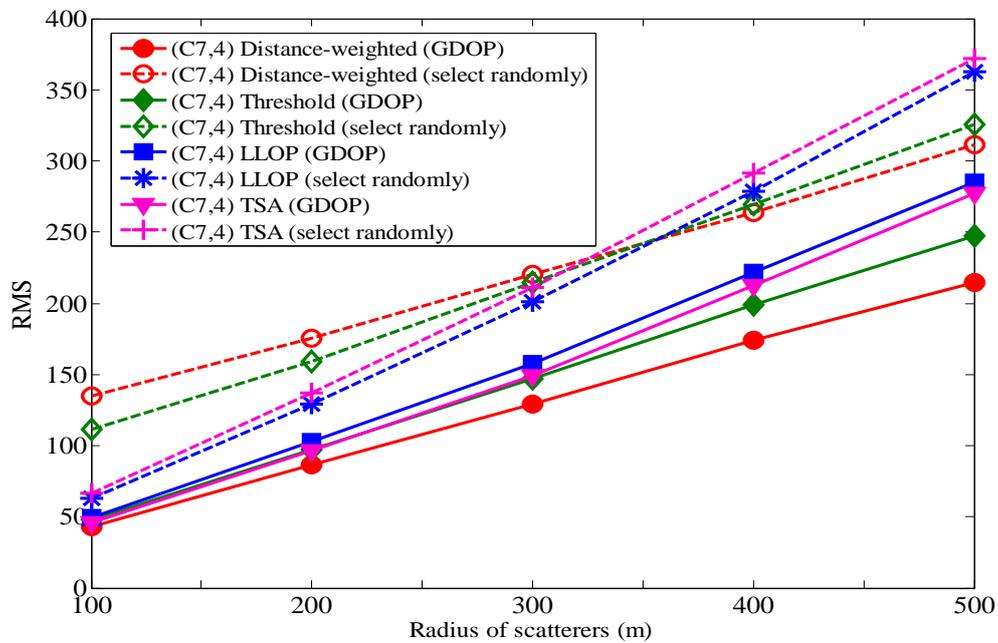
**Fig. 2.** Average location error versus the disc radius of CDSM.
