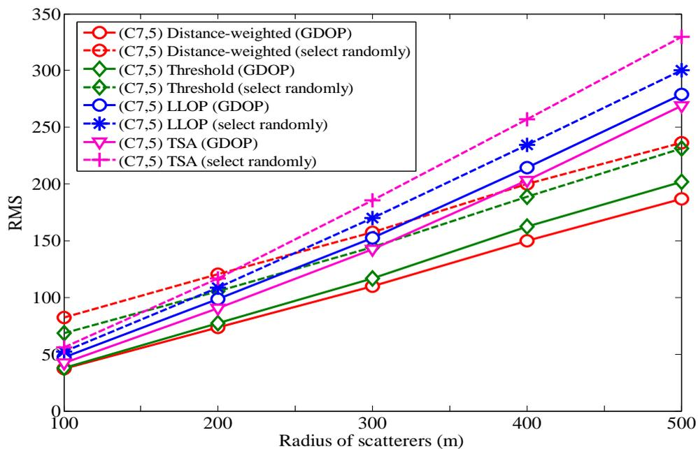
**Fig. 3.** Comparison of RMS errors when NLOS errors are modeled as CDSM.
