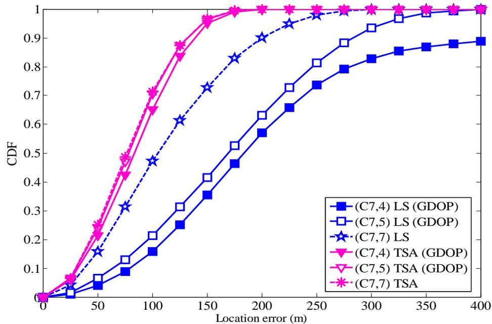
Fig. 7. Comparison of error CDFs when the subset with minimum GDOP and using all seven BSs.
