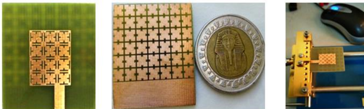
Fig. 11. The fabricated antenna and measurement setup
