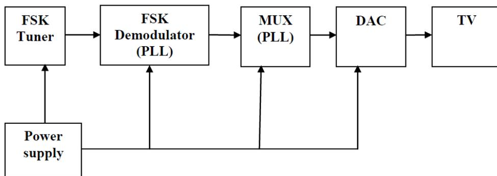
Figure 1: Block diagram of decoder.
