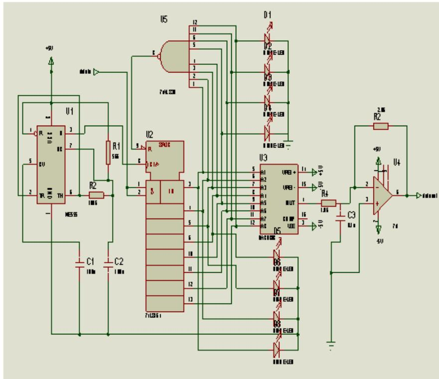
Figure 7: Schematic diagram of the shift register connected the DAC.
