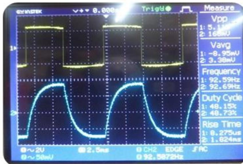
Plate 1 (b): Input digital signal at a frequency of 92.59 Hz compared to the digital signal from the demodulator output after filtering and before signal conditioning
