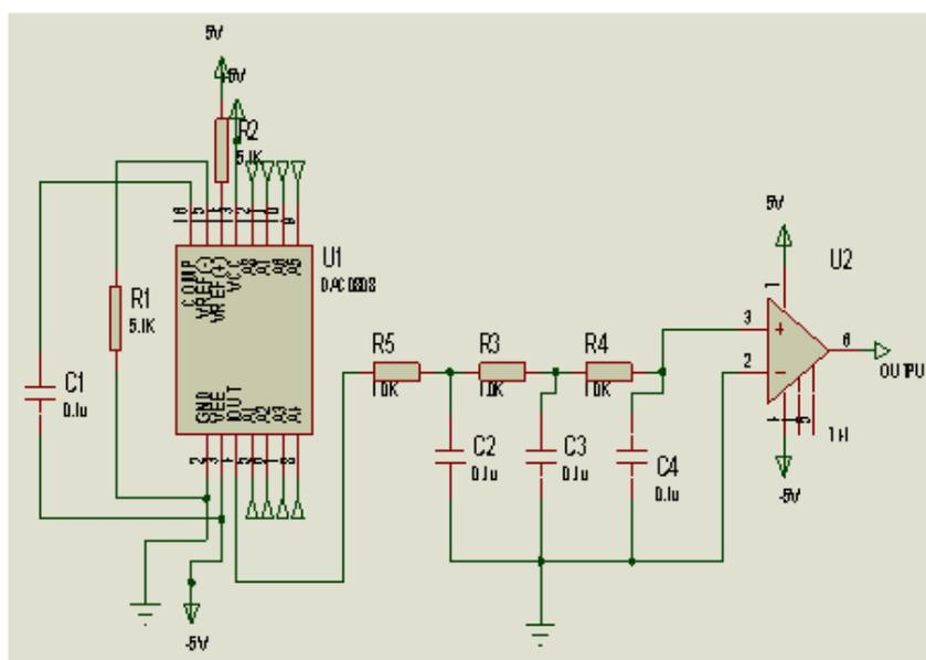
Figure 6: Schematic diagram of the 8 bit data conversion circuit.
