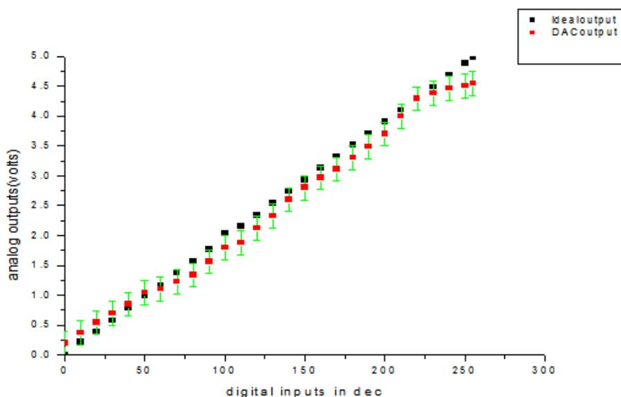
**Figure 9:** A correlation between the analog outputs to the digital inputs of the decoder.
