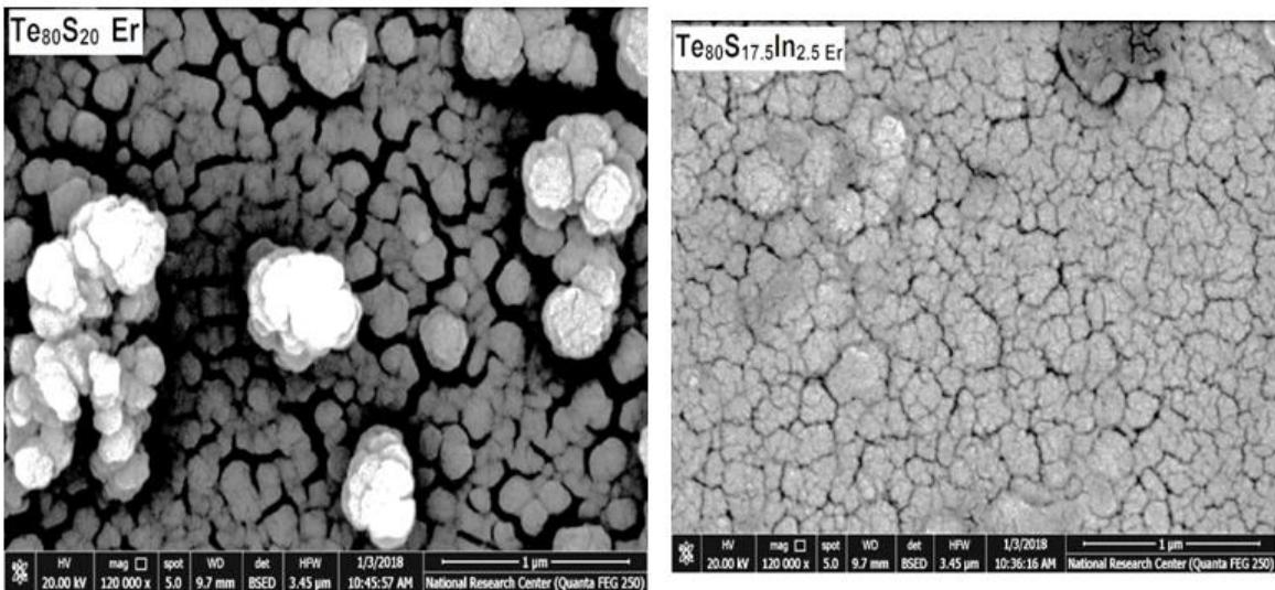
**Fig [3]** scanning electron micrograph image of chalcogenide system  $\text{Te}_{80}\text{S}_{20-x}\text{B}_x$  where ( $x=0,2.5,5$  and  $\text{B}=\text{In}$  or  $\text{As}$ ) thin films
