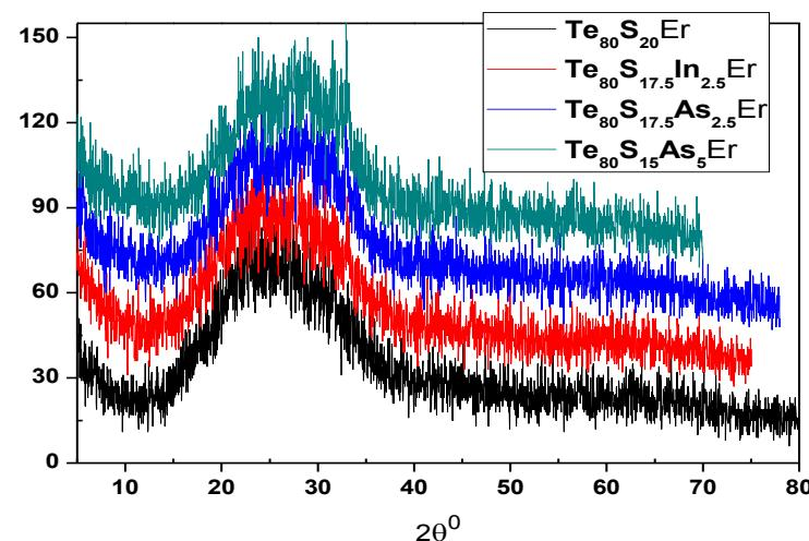
Fig [2] X-ray diffraction patterns of system  $\text{Te}_{80}\text{S}_{20-x}\text{B}_x$  where ( $x=0, 2.5, 5$  and  $B=\text{In}$  or  $\text{AS}$ )thin film covered with Er layer.
