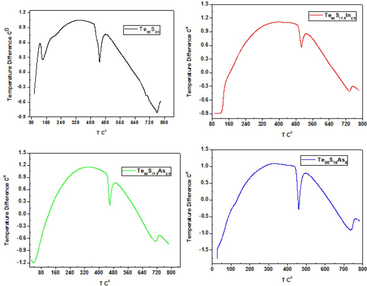
**Fig [5]** DTA thermograms of chalcogenide system  $\text{Te}_{80}\text{S}_{20}-\text{xBx}$  where ( $x=0,2.5,5$  and  $B=\text{In}$  or  $\text{As}$ ).
