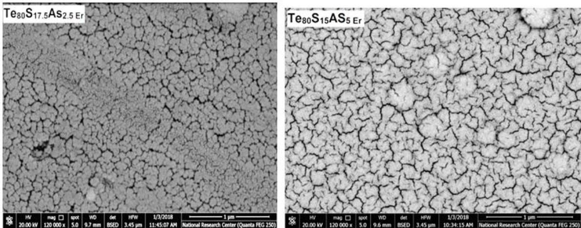
**Fig [4]** scanning electron micrograph image of chalcogenidesystem  $\text{Te}_{80}\text{S}_{20-x}\text{B}_x$  where ( $x=0,2.5,5$  and  $\text{B}=\text{In}$  or  $\text{As}$ ) thin film cover with Er layer.
