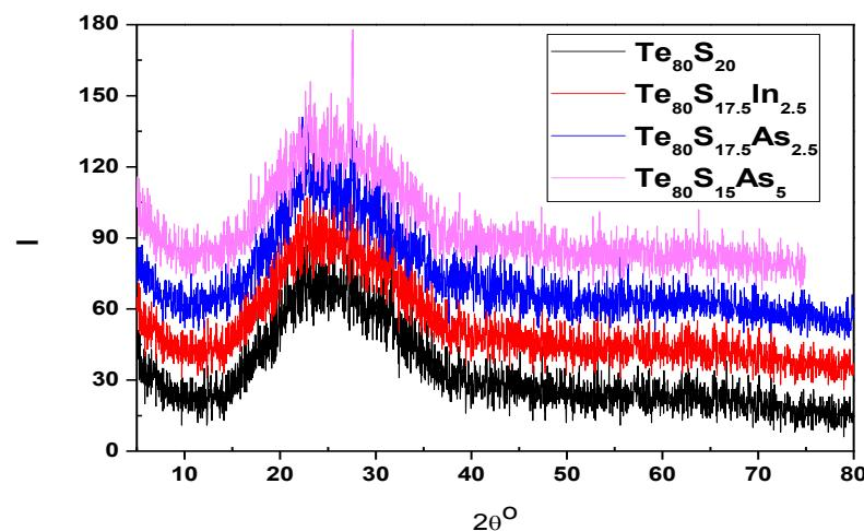
Fig [1] X-ray diffraction patterns of system  $\text{Te}_{80}\text{S}_{20-x}\text{B}_x$  where ( $x=0, 2.5, 5$  and  $B=\text{In}$  or  $\text{AS}$ )thin film deposited on a glass substrate.
