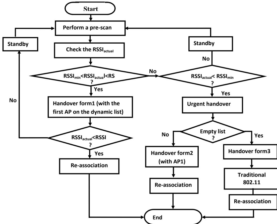
Figure 3: Prevent Scanning Process Flowchart
