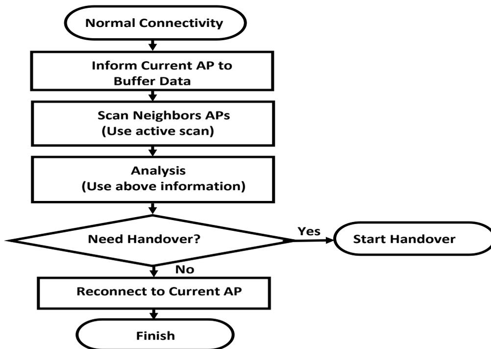
Figure 1: Proactive Scanning Phase Flowchart
