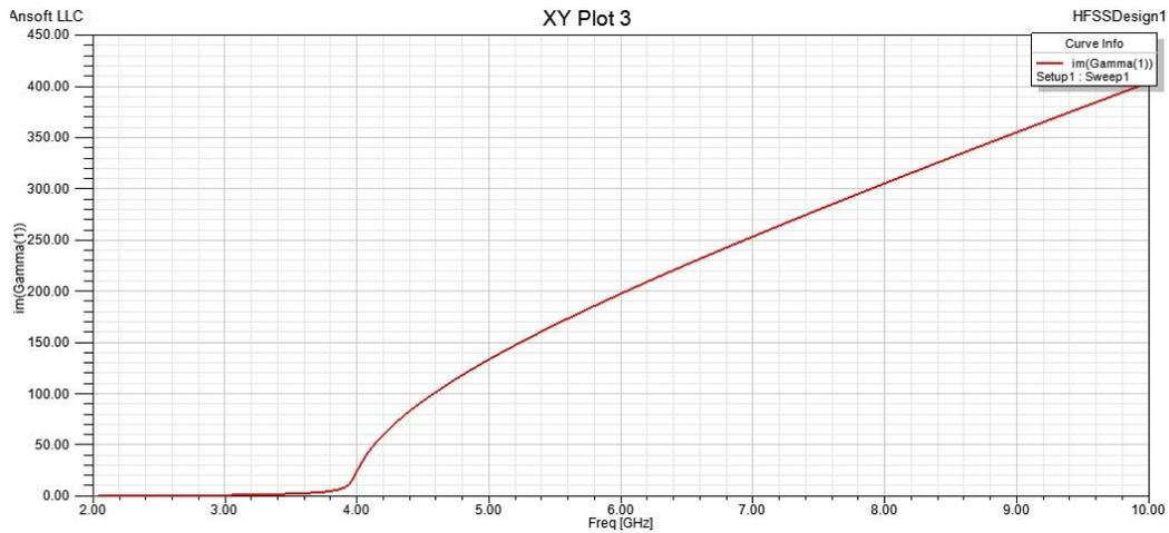
**Fig. 6 Phase Constant of Designed SIW**
