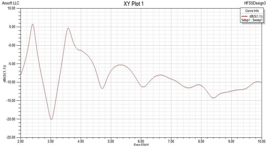
**Fig. 8  $S_{11}$  Vs Frequency curve of the SIW Leaky Wave Antenna**
