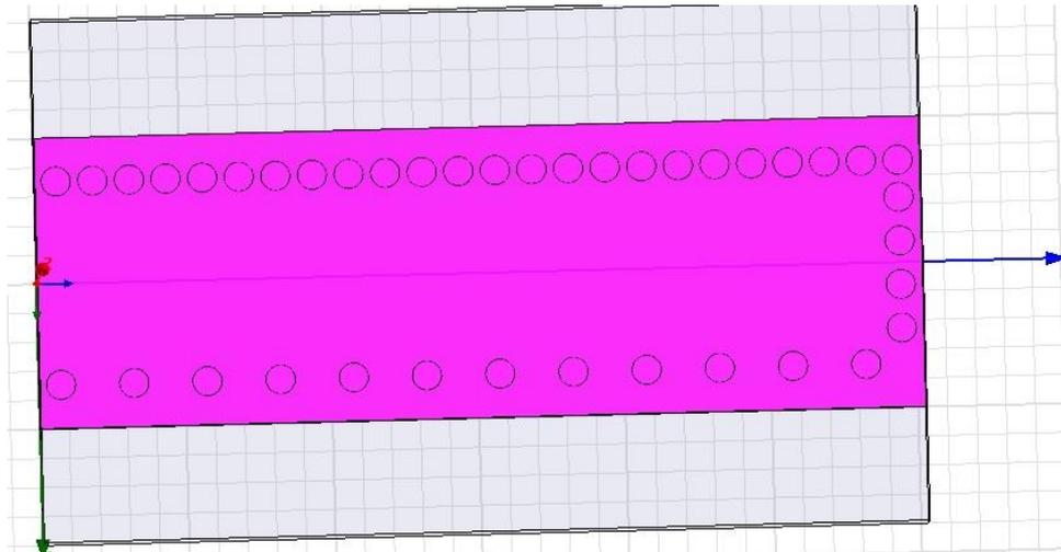
Fig.3 SIW leaky Wave antenna
