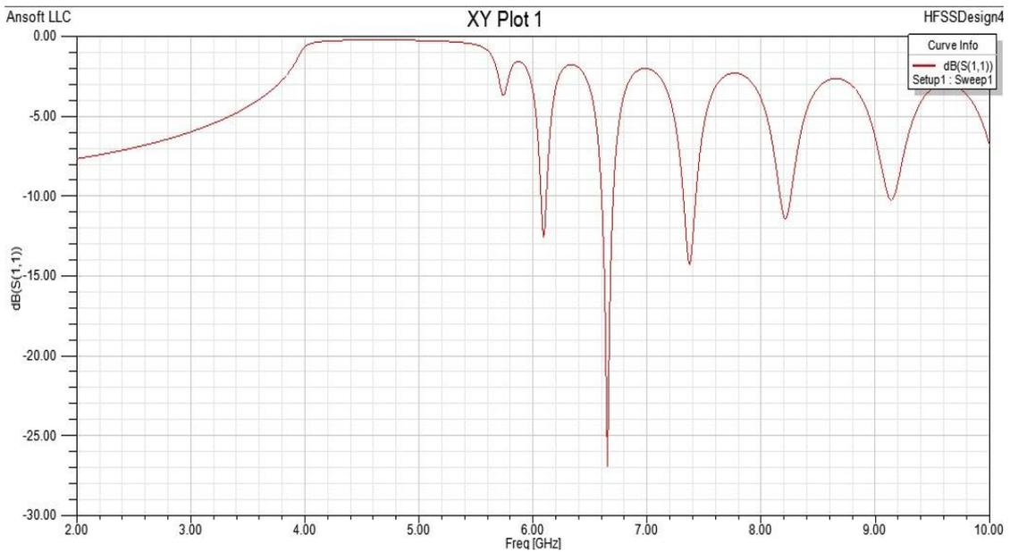
**Fig. 9  $S_{11}$  Vs Frequency curve of the SIW Leaky Wave Antenna**
