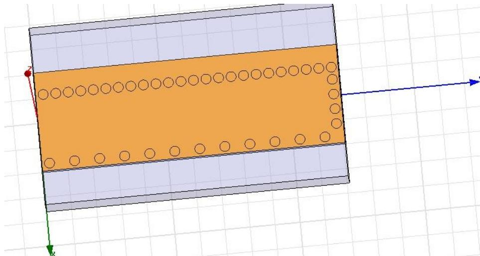
Fig.4 SIW leaky Wave antenna with radiating slot towards the edge
