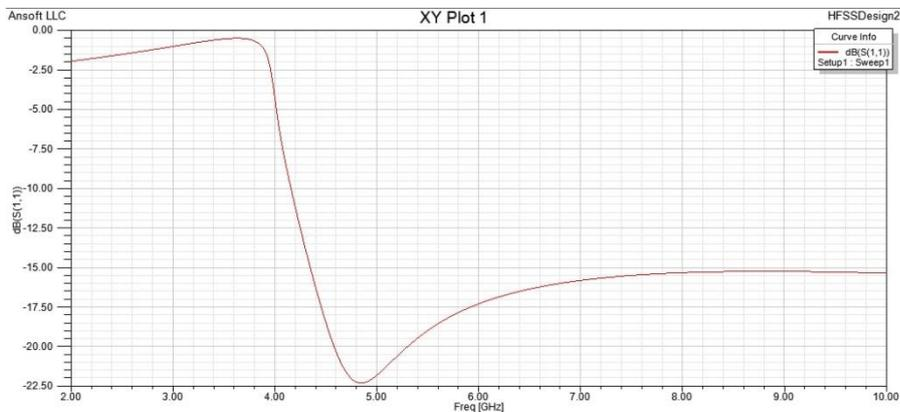
**Fig. 7 S<sub>11</sub> Vs Frequency curve of the SIW slotted Antenna**
