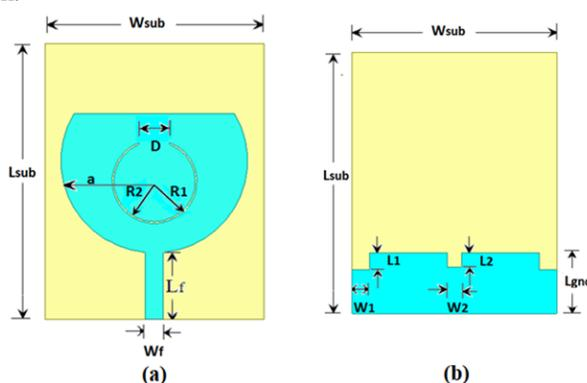
**Fig.1. Design of the proposed modified circular-shaped printed monopole antenna with the circular arc slot.**
