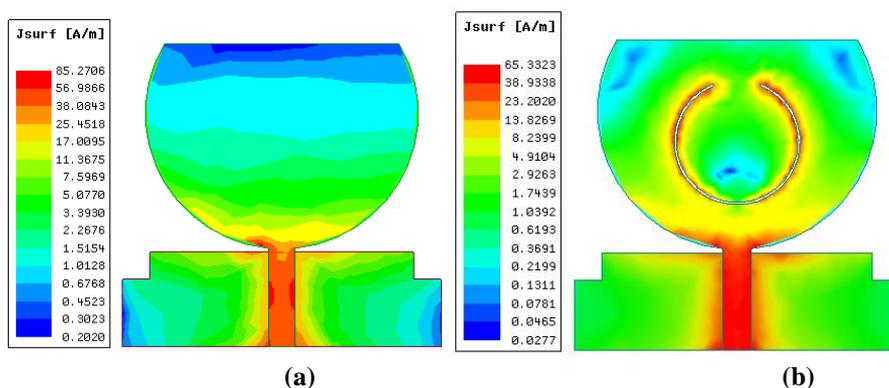
Fig.4. Antenna Current Distribution at 2.44 GHz; (a) without slot, (b) with the slot.
