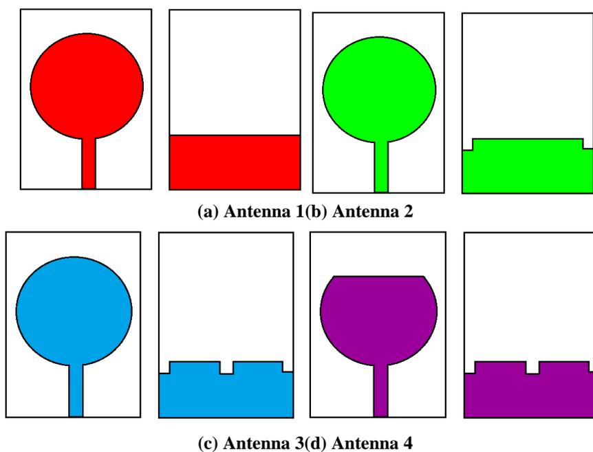
Fig.2. Development of modified circular-shaped UWB monopole antenna.
