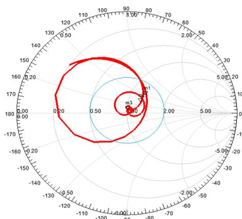
**Fig.13. Simulated Smith chart of Dual-band Antenna**
