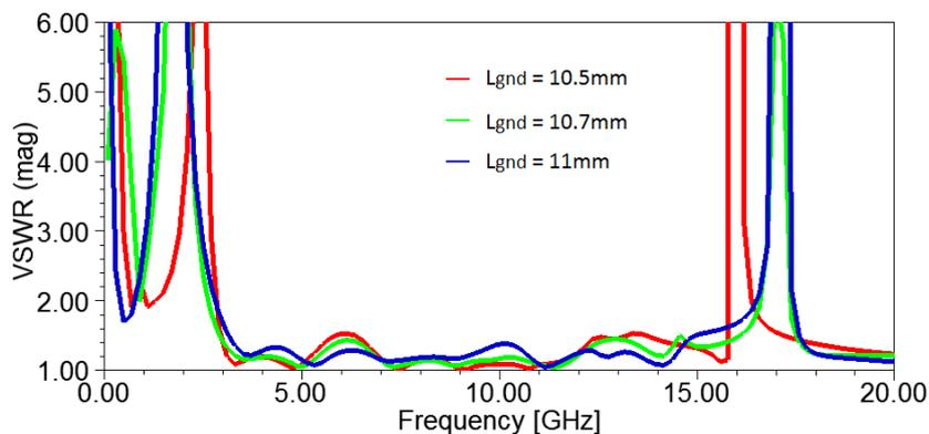
Fig.5 VSWR plots for the variation in length  $L_{\text{gnd}}$ .
