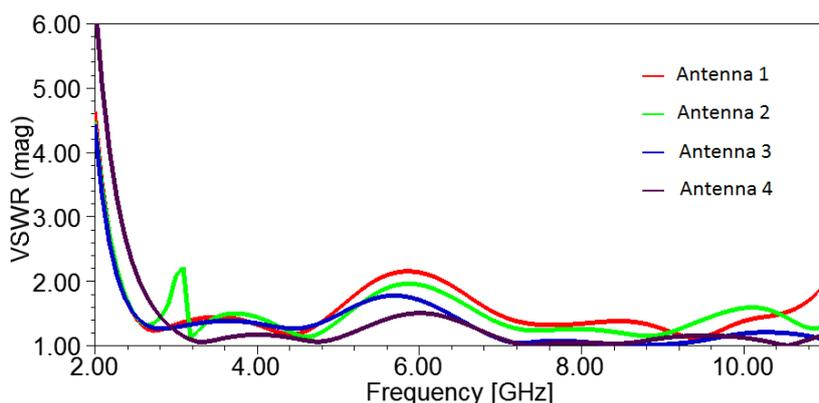
Fig.3 VSWR plots for UWB evolution antenna designs.
