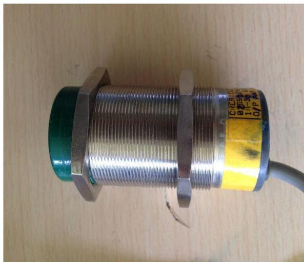
Metal plates are fitted on the edge of the base at where the charkhas are placed at that side. Third metal detector is fitted on the bottom side of the trolley and nearer to base. It detects the metal plates and giving the order to proxy sensor for the activatio
