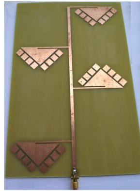
Fig.8. Fabricated antenna design
