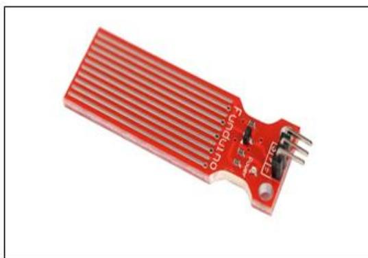
**Fig.2** Water level sensor
