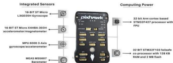
Fig 2.1 Pixhawk 2.4.8 flight controller
