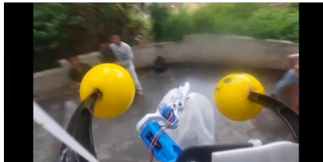
fig. 2 drone with the robotic arm holding a cover
