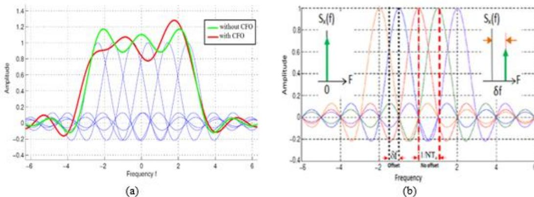
Figure 2. Simple concept of the effects of frequency offset (left) OFDM spectrum (right) OFDM signaling [12]
