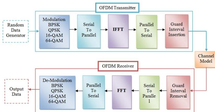
Figure 1. General diagram of OFDM including important stage.
