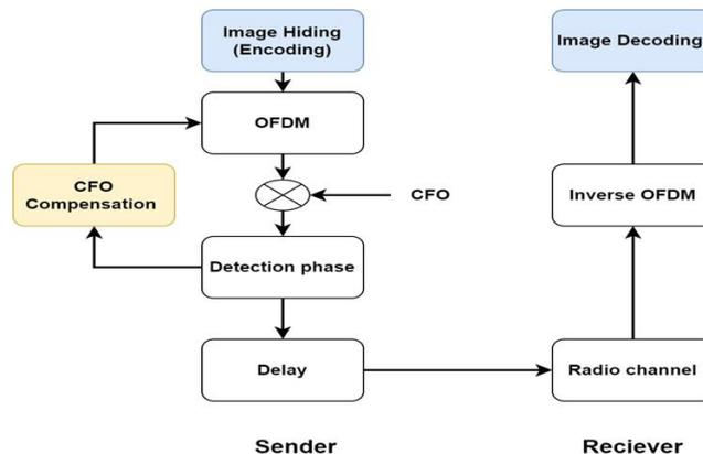
Figure 3. Proposed CFO compensation of an OFDM system
