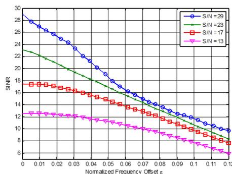
FIGURE 6. Signal-to-Interference-Noise-Ratio (SINR) performances over CFO.
