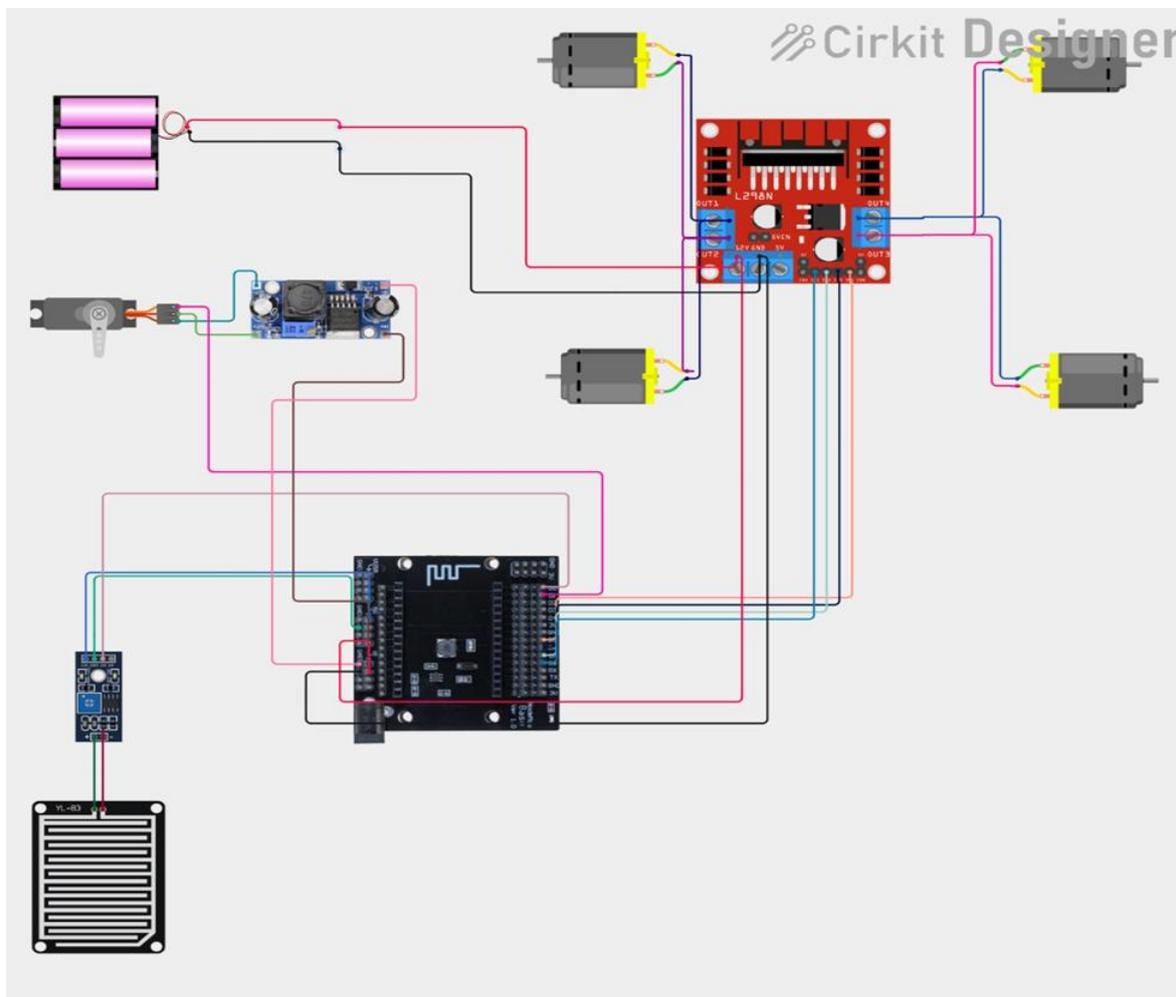
**Figure. 3.3 Interconnection of components embedded together**
