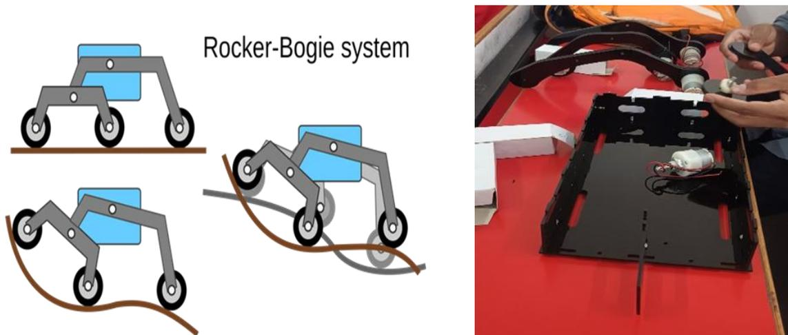
Figure. 3.1 Design, Analysis and Fabrication of Rocker Bogie Mechanism
