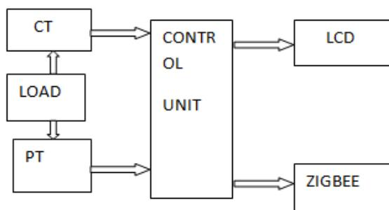
**Fig- ENERGY METER AT SUBSCIBER END**
