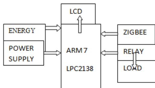
Fig1-Transmitting Section of System
