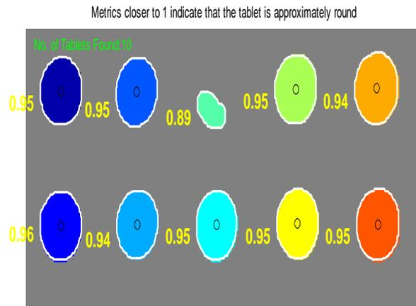
Figure 6 Defected tablet found
