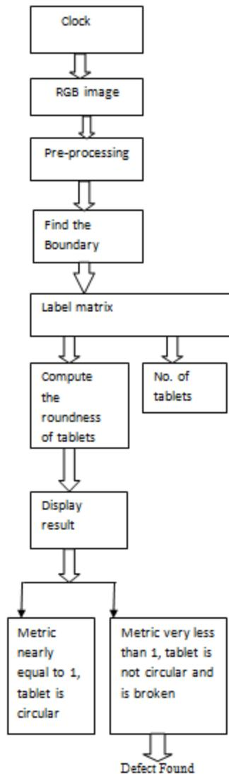
Figure 3 Block diagram shows how to find the defect
