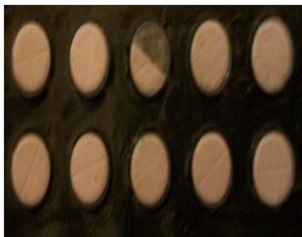
Figure 1 Different tablet packet with defect
