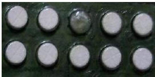
Figure 7 Tablet packet with missing tablet
