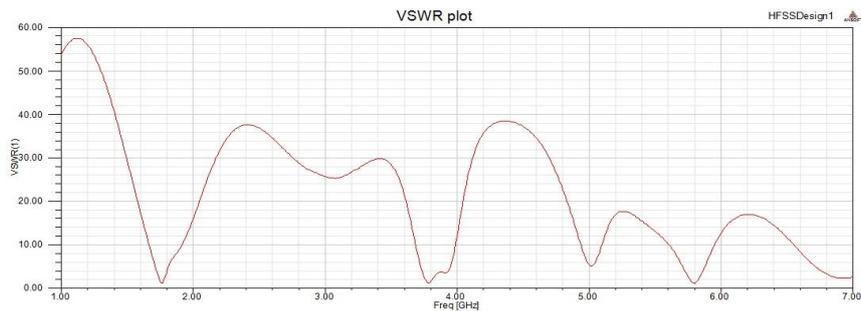
Figure 9. VSWR plot for the basic antenna
