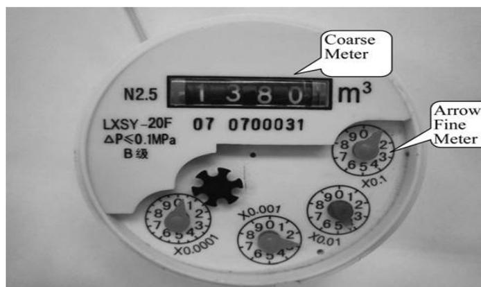
Fig.1 Mechanical Water Meter
