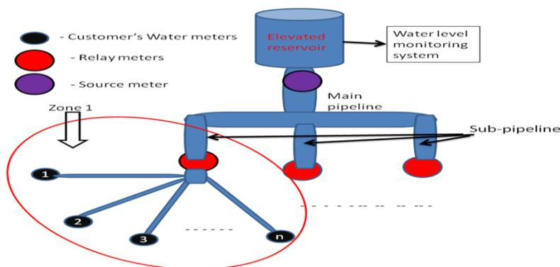
Fig.7 Water Leakage Detection System
