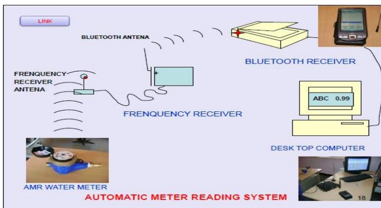
Fig.2 Automatic meter reading system
