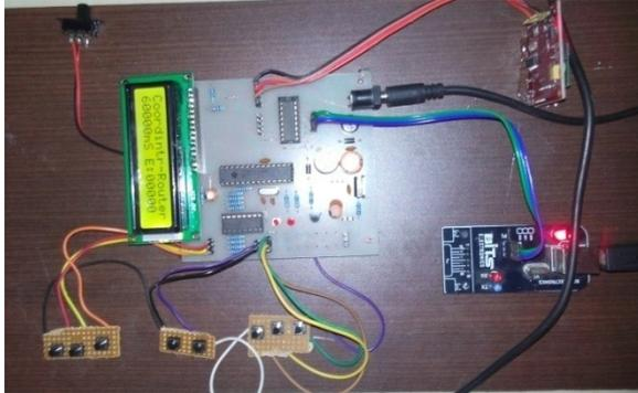
Fig4.2(a) Sensor node designed which is configured as coordinator
