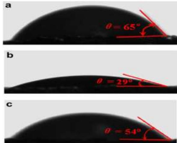
Fig 6Static contact angles of droplet on different surfaces: (a) pure water droplet on clean surface boiled in pure water,  $\theta = 65^\circ$ ; (b) SiO<sub>2</sub>/water nanofluid droplet on silica nanoparticles-deposited surface at the evaporator,  $\theta = 29^\circ$ ; and (c) Al<sub>2</sub>O<sub>3</sub>/water nanofluid droplet on alumina nanoparticles-deposited surface at the evaporator,  $\theta = 54^\circ$ [26].
