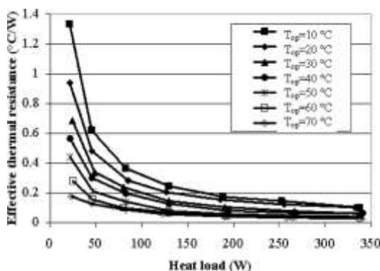
Fig 3 Thermal resistance at various heat loads and operating temperatures[20]
