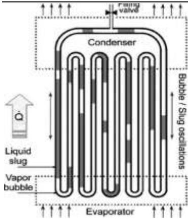
Fig 1 Schematic of a Pulsating Heat Pipe[3] .
