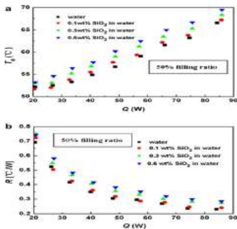
Fig. 5 Thermal performance of the PHP/OHP charged with SiO<sub>2</sub>/water nanofluids at different mass concentration(a) Average evaporator temperature; (b) overall thermal resistance[26].
