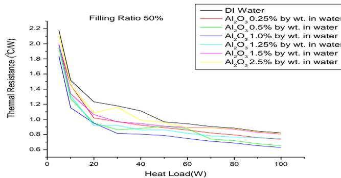
Fig 7 Effect of concentration of Al<sub>2</sub>O<sub>3</sub> on thermal resistance of PHP at FR 50%[49]
