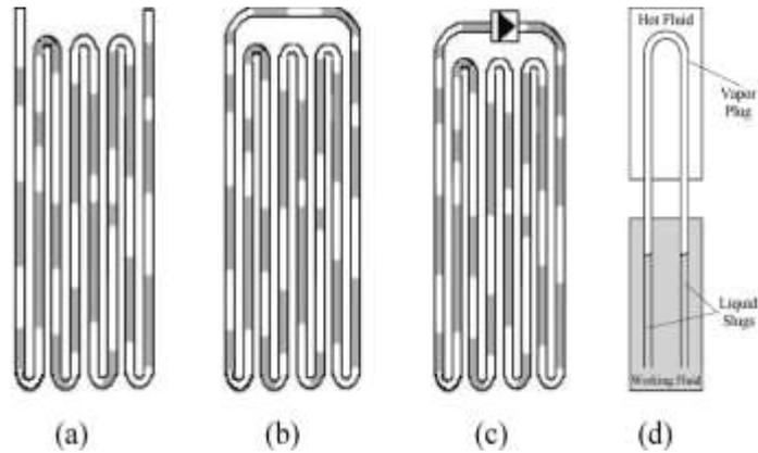
Fig 2 Different PHPs: (a) closed-end, (b) closed-loop, (c) closed-loop with check valve, and (d) PHP with open ends[16]
