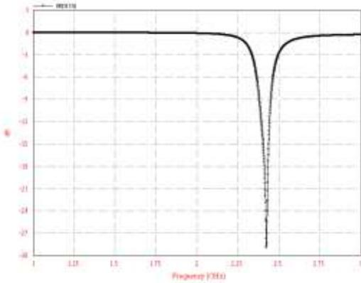
Fig. 2: Gain Vs frequency of rectangular antenna
