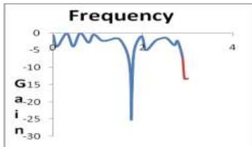
Fig.11: Practical graph (Gain Vs frequency of slotted antenna) by excel.
