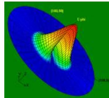
The simulated 2D H plane radiation pattern of simulated antenna for 9.54 GHz is shown in fig 6. The simulated E plane radiation pattern (3D-view) of Slotted Antenna for 9.54 GHz is shown in fig 7. The simulated H plane radiation pattern (3D-view) of Slotted Antenna for 9.54 GHz is shown in figure 8.
