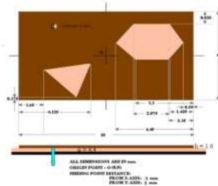
Figure 2: Simulated Antenna configuration
