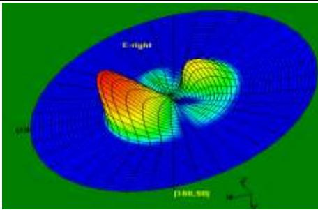
Figure 11: E-Plane (3D View) Radiation Pattern for slotted antenna at 12.90 GHz
