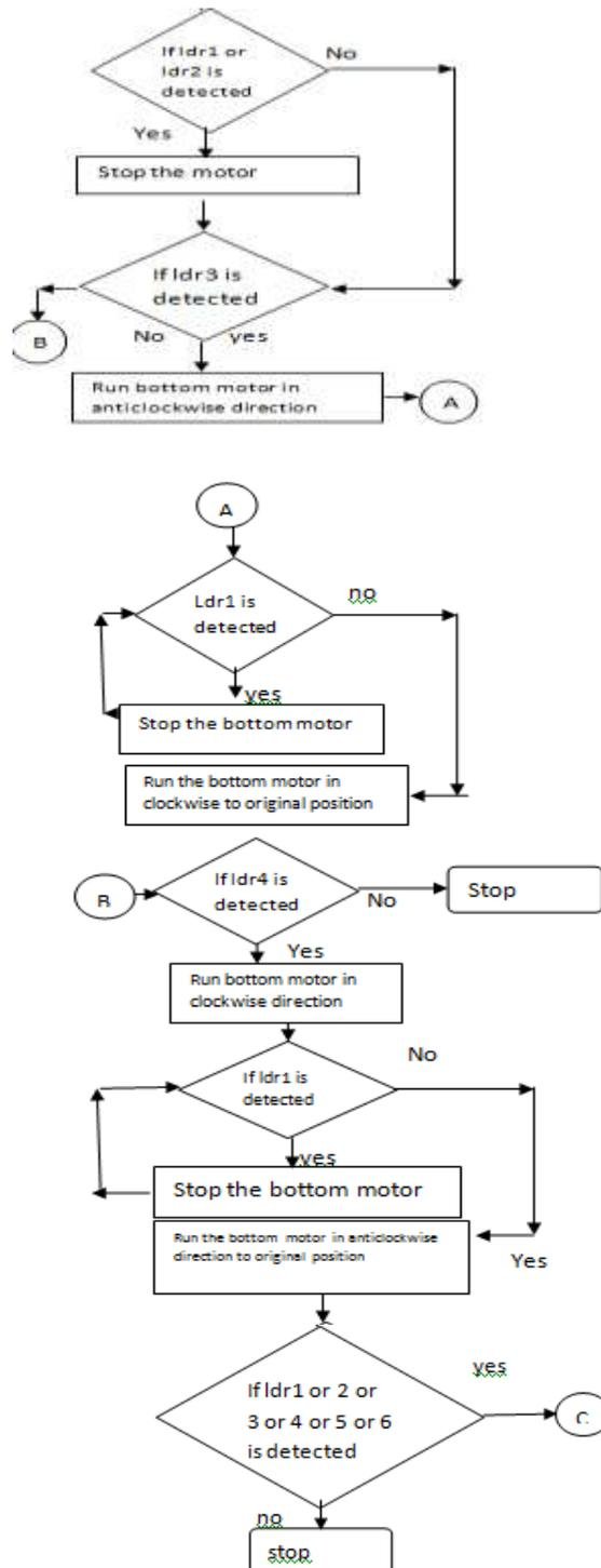
Fig 6. Flow chart of sun tracking system
