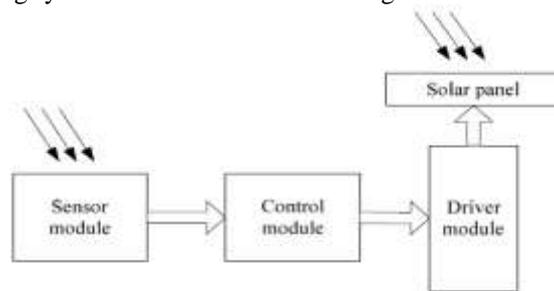
fig 1. Sun tracking system structure
