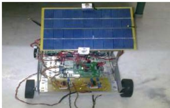
Fig 6. Prototype of “advanced sun tracking system on wheels”
