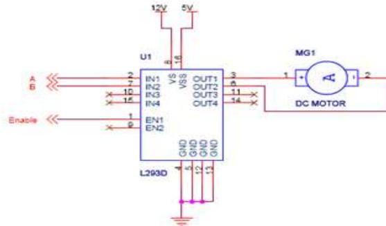
Fig.5. L293D dc motor driver circuit
