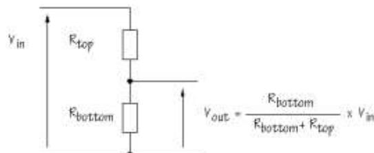
Fig 3.Voltage divider circuit
