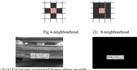
Fig.5 (A) Car images segmented license plates on right
