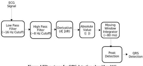
Figure 4 Filter stages for QRS detection algorithm [11]
