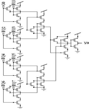
Figure 9. Schematic of AND Gate Y0 of Modified 64-Bit Binary Comparator
