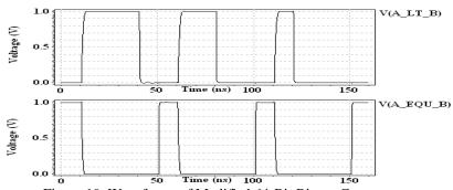
Figure 19. Waveforms of Modified 64-Bit Binary Comparator
