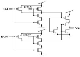
Figure 13. Schematic of AND Gate Y4 of Modified 64-Bit Binary Comparator
