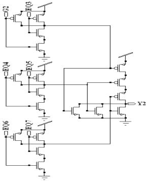
Figure 11. Schematic of AND Gate Y2 of Modified 64-Bit Binary Comparator
