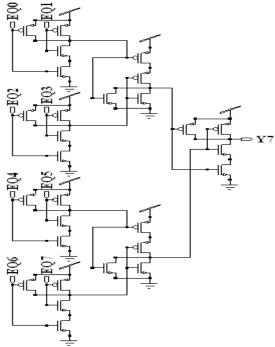
Figure 17. Schematic of NAND Gate YE of Modified 64-Bit Binary Comparator
