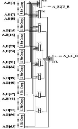
Figure 18. Schematic of Modified 64-Bit Binary Comparator
