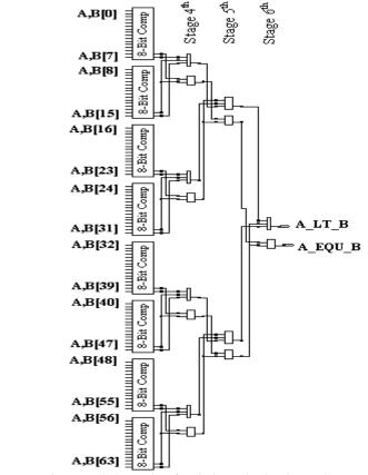
Figure 6. Schematic of Existing 64-Bit Binary Comparator
