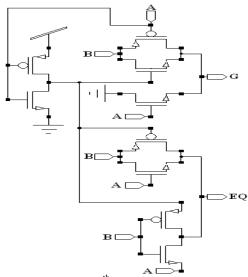
Figure 3. Schematic of Stage 0<sup>th</sup> of Existing 64-Bit Binary Comparator
