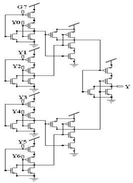
Figure 16 Schematic of NOR Gate YL of Modified 64-Bit Binary Comparator
