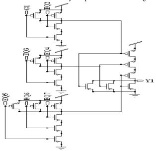
Figure 10. Schematic of AND Gate Y1 of Modified 64-Bit Binary Comparator
