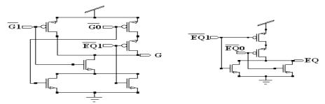
Figure 5. Schematic of Stage 2<sup>nd</sup> of Existing 64-Bit Binary Comparator
