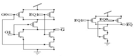
Figure 4. Schematic of Stage 1st of Existing 64-Bit Binary Comparator
