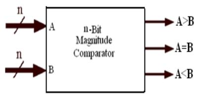
Figure 1. Block Diagram of n-Bit Magnitude Comparator
