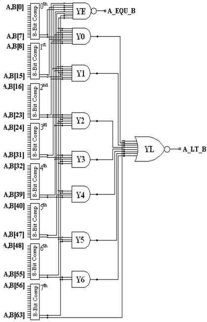
Figure 8. Logic Diagram of Modified 64-Bit Binary Comparator
