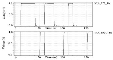
Figure 7. Waveforms of Existing 64-Bit Binary Comparator
