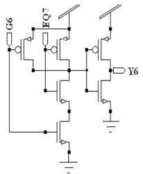
Figure 15. Schematic of AND Gate Y6 of Modified 64-Bit Binary Comparator
