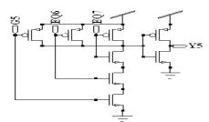
Figure 14. Schematic of AND Gate Y5 of Modified 64-Bit Binary Comparator
