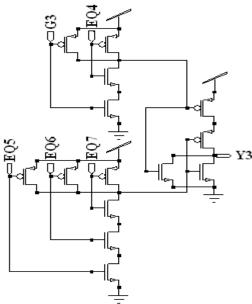
Figure 12. Schematic of AND Gate Y3 of Modified 64-Bit Binary Comparator
