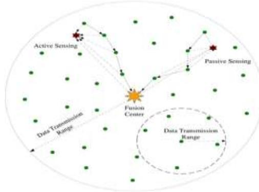
Fig. 1. Routing in WSNs for signal detection
