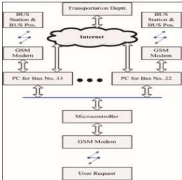
Figure 5. Block Diagram of BASE Station Module
