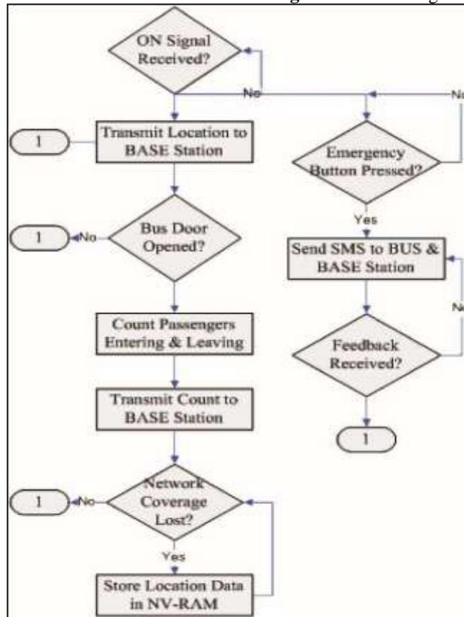
Figure 4. Flow Chart for In-BUS Module
