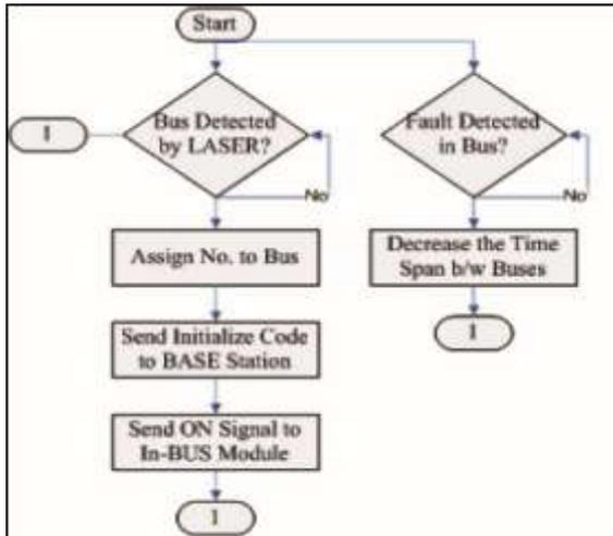
Figure 2. Flow Chart of BUS Station Module
